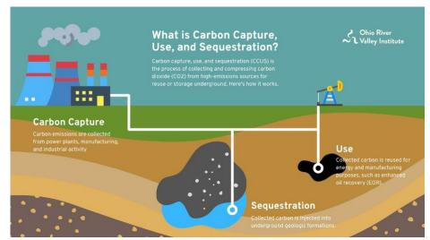
But what does CCUS "carbon capture utilization and storage" mean? It is a mechanical and chemical technology to capture the carbon emissions from the smoke stacks of high emitting power plants and industrial facilities. The captured carbon is in the form of CO2. It is compressed and manipulated so it can be transported to a site where it can be used by industry or sequestered permanently in the ground.
